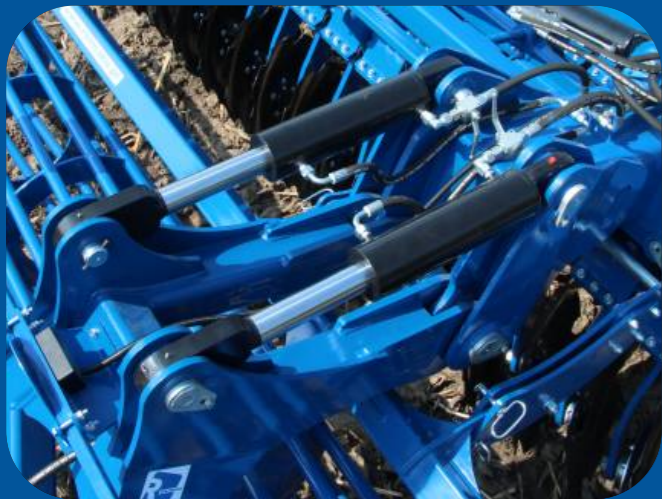
The arms blocking system is controlled by the hydraulic cylinder, which ensures safety during transportation.
