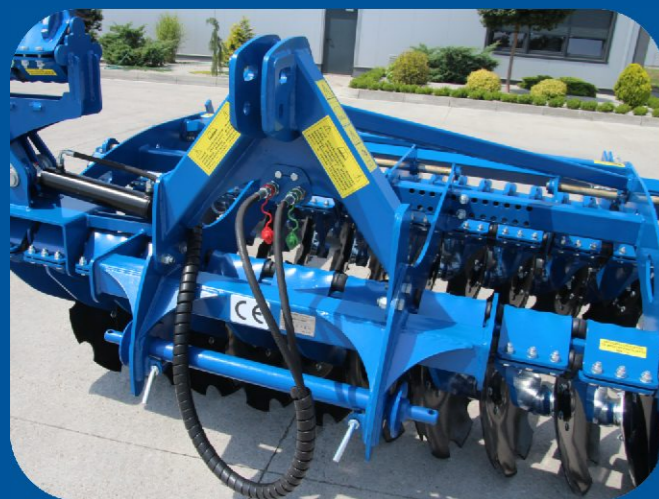
Bidirectional hydraulic cylinder responsible for folding two discs of working section.
