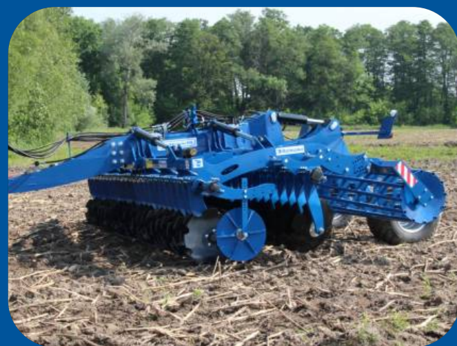
Adjustable rear beam with discs - changing the rear beam towards the front one is quick and easy to use.
