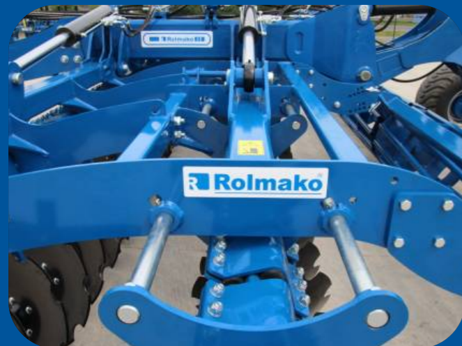
Adjustable rear beam with discs - changing the rear beam towards the front one is quick and easy to use.
