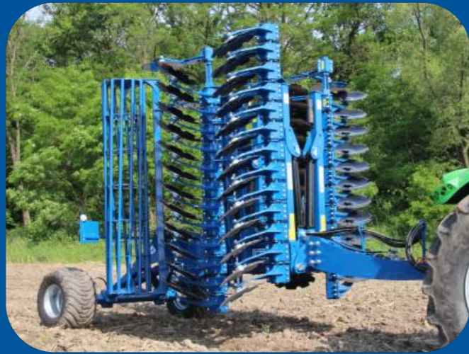
The arms blocking system is controlled by the hydraulic cylinder, which ensures safety during transportation.
