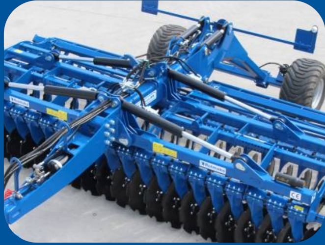
Harrow's arms are folded by 4 massive hydraulic cylinders. Two of them are protected against unwanted fall-down by the hydraulic locks.
